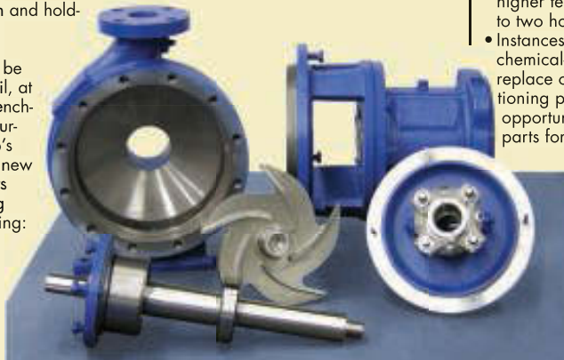
FIGURE 2. Major components can be laid out for inspection
