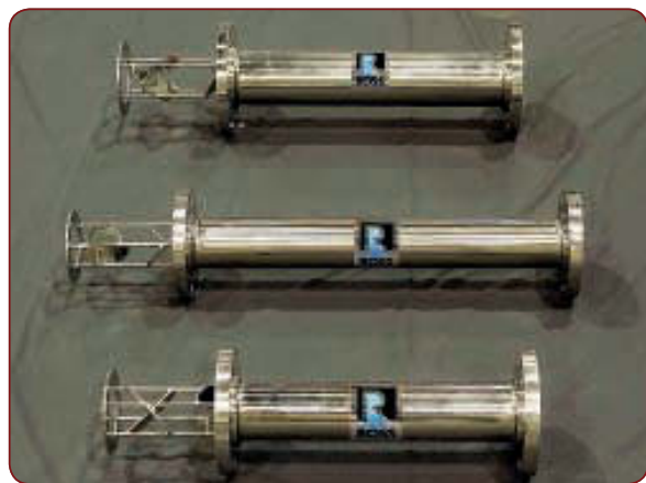
Shown are removable LPD mixing elements supplied with a retain ring which goes between two mating flanges to keep the mixer from spinning or moving downstream
