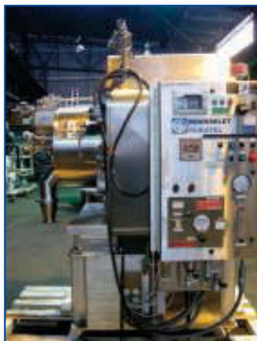
500mm X 250mm Rousset Robotel Peeler Centrifuge, Hastelloy C22
